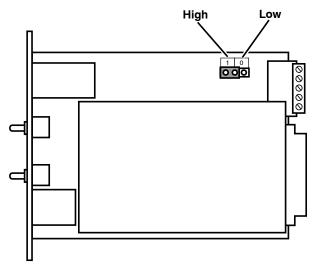
Figure 7.2: Control Module Jumper
